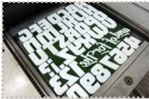
Vandercook SP15 with the new laser type blocks locked-up
