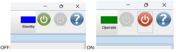
**YOU MUST TURN ON THE CMS BEFORE STARTING THE LC SYSTEM!** If you turn on the LC without the CMS on, you will flood the source and potentially damage the instrument. You will be required to write a guide on how to clean a flooded source to show other students how to fix this mistake.
