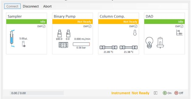
9. Verify there is fluid in the bottles on top of the LC stack. Determine if you are going to be using acid in your mobile phase or not. **Organometallic complexes should NOT** be analyzed with acid in the mobile phase, so use bottles A2 and B2. All others use acid and bottles A1 and B1. If the mobile phase volume is less than 200 mL, ask Dr. Boersma for more.
