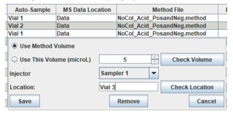
19. You know your vial number by where you placed your sample in the autosampler. Vial number 1 is always a blank and is in the front right position nearest you. That column is vials 1 to 10. The column to the right is vials 11 to 20. The next column is 21 to 30 and so on. Vial 81 is the autosampler wash vial. Make sure there is solution in Vial 1 and 81. There are solvents on the bench to the right to fill these vials with.
