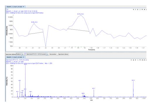
29. You can find your desired ion by right clicking inside the spectra to zoom to the region of interest. Then right click and drag below the m/z axis (x-axis) and the region in which the m/z will appear in the chromatogram.
