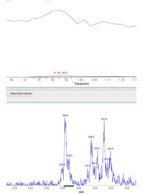
Here you can see that 540.8 is a contaminant in the blank injection. So a new wash solution should be added to vials 1 and 81. You can export your data as a .pdf or copy the data to your box folder and view at your leisure via your own copy of the software.
