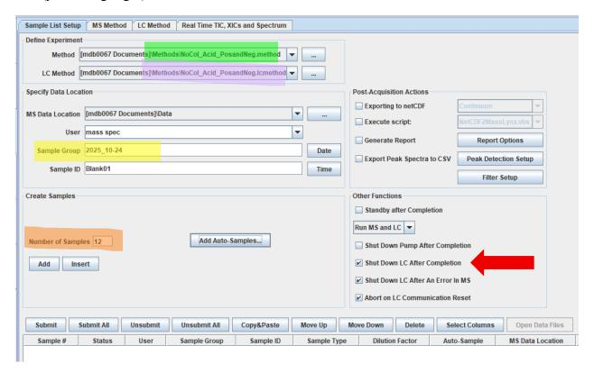
In the Define experiment box click the ... by method to select the mass spec method (green highlight). Then click the ... to define the LC method (purple highlight). Acid should be used UNLESS your sample is an organometallic complex.
