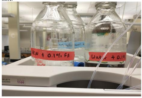
There must be adequate mobile phase on the system or you risk damaging the LC pump!!
