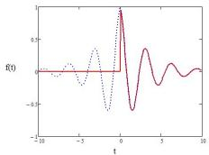
Fig.1. Two types of exciting pulses: the solid curve is the exponential pulse, the dotted line is the double exponential pulse;  $\omega = 2, \tau = 3$
