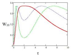
t Fig.3. Dependence of the probability of excitation of a quantum oscillator by a double exponential pulse (2) at the 0→1 transition on the pulse duration for different Rabi frequencies: solid curve -  $\Omega_0$ =2, dotted line -  $\Omega_0$ =3, dashed curve -  $\Omega_0$ =4;  $\omega_0$ =5,  $\omega_0$ =5.5
