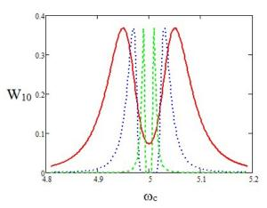
Fig.5. Excitation spectrum of a quantum oscillator by a double exponential pulse with different duration at the  $0 \rightarrow 1$
