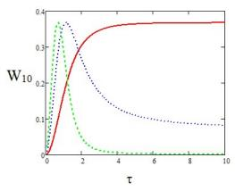
Fig.2. Dependence of the probability of excitation of a quantum oscillator by an exponential pulse (1) at the  $0\rightarrow 1$  transition on the pulse duration for different Rabi frequencies: solid curve -  $\Omega_0=1$ , dotted line -  $\Omega_0=2$ , dashed curve -  $\Omega_0=3$ ;  $\omega_0=5$ ,  $\omega_c=5.5$ When a quantum oscillator is excited by a double exponential pulse (2) in the case of a weak perturbation
