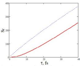
Fig.4. Integral fluorescence signal in sodium vapor as function of pulse duration calculated with the use of different approaches (resonance case): solid line – generalized kinetics model, dotted line – standard approach; t=240 fs,  $\omega_0 = 2.013$  eV,  $\Omega_0 = 0.0272$  eV
