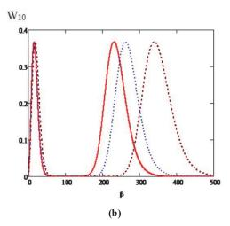
Fig.2. Excitation probability of transition  $0 \rightarrow 1$  in quantum oscillator as function of dimensionless pulse duration ( $\beta$ ) for weak field  $-E_0=10^{-3}$  a.u. (a), strong field  $-E_0=0.04$  a.u. (b) and different values of dimensionless chirp: solid line  $-\alpha=0$ , dotted line  $-\alpha=0.5$ , dashed line  $-\alpha=1$
