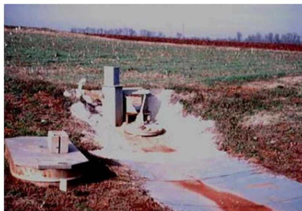
Runoff volume was monitored by 0.305 meter H-flumes equipped with runoff hydrograph recorders. A model N-1 Coshoc-ton-Type runoff sampler and runoff storage tank were used for runoff sample collection.
