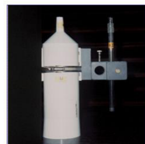
NH 3 Sampler (Leuning et al., 1985) and Glass Tube Cost: US$250.00 versus US$1.35
