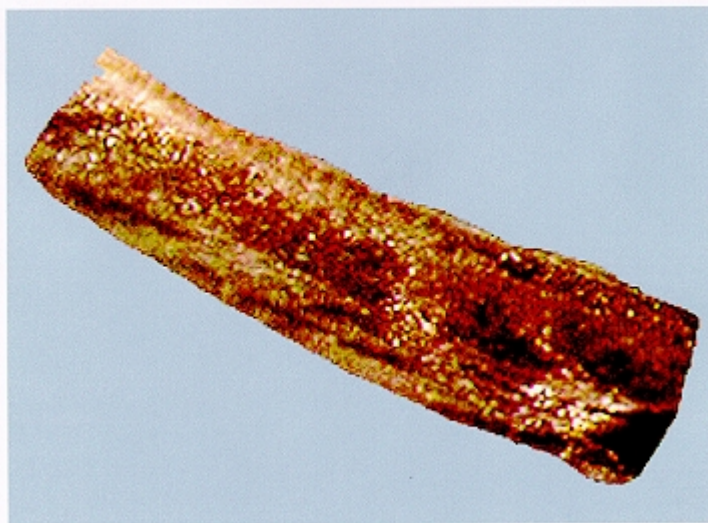
Figure 1b. PVA/PAA fibers containing \text{AgNO}_3 after irradiation.
