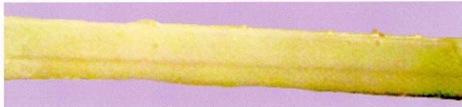
Figure 1a. Poly (vinyl alcohol) fibers, PVA, crosslinked with dimethylsulfoxide in the presence of poly (acrylic acid), PAA.
