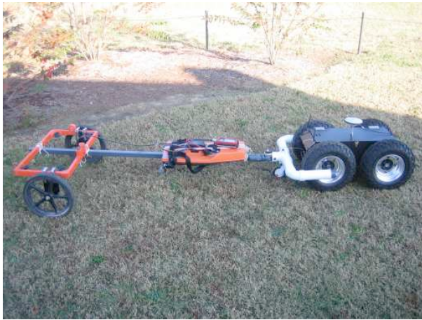
Fig. 2. Segway robot and geophysical instrument trailer
