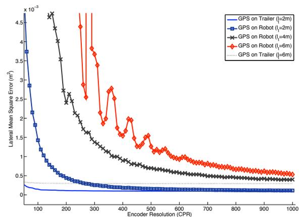
Fig. 7. Control System Performance for Varying Encoder Resolutions
