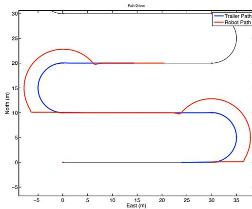
Fig. 9. Simulation Result: GPS on Trailer &  $l_t = 6m$
