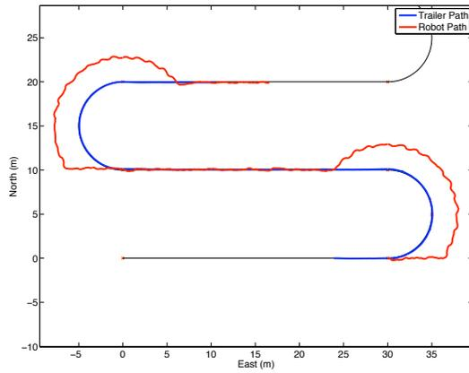
Fig. 8. Simulation Result: GPS on Robot &  $l_t = 6m$
