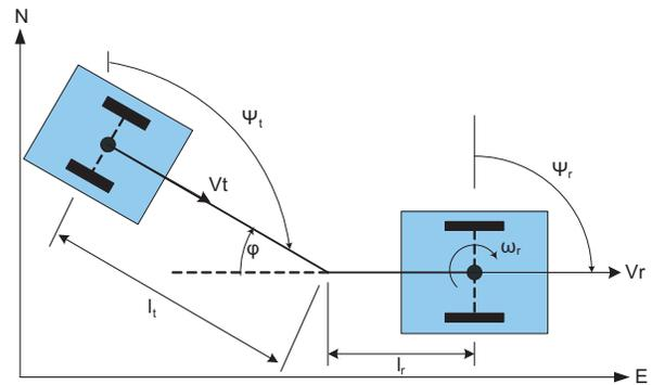
Fig. 3. Schematic Representation of Segway and Trailer
