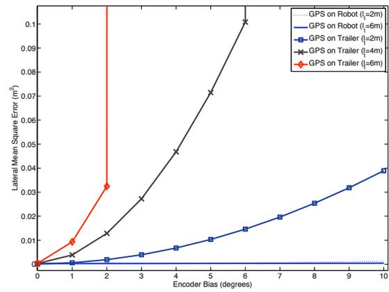
Fig. 11. Control System Performance for Varying Encoder Biases
