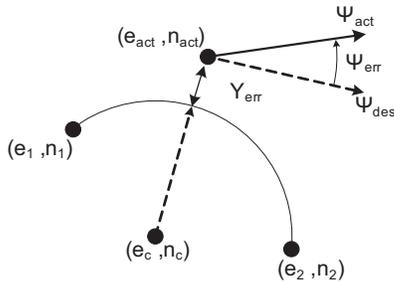
Fig. 5. Arc Segment Errors
