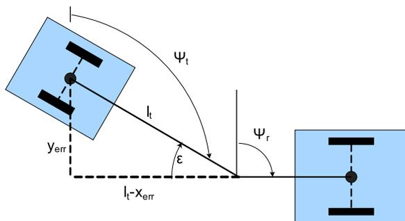
Fig. 6. Effect of Hitch Angle Error on Error States
