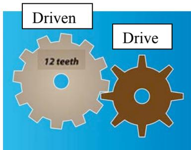
This is a gear train. A gear train consists of a drive gear that is connected to a motor and a driven gear that is being moved by the drive gear. In this picture, the small brown gear is the drive gear; it has 8 teeth. The gray gear is the driven gear; it has 12 teeth. To determine the **gear ratio** of this system we divide the number of teeth of the driven gear by the number of teeth of the drive gear. **Driven/Drive**.
