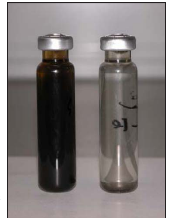
Visual comparison of the stability of Auburn's nanoparticles (left) vs. unstabilized particles (right) after five days
