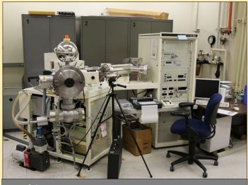
One of the new multi-collector thermal ionization mass spectrometers (MAT-262).
