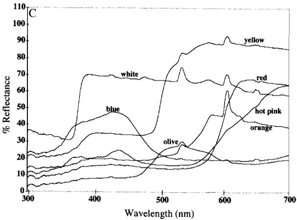
from the surface of the band relative to a 99% Spectralon white reflectance standard. For each band, 20 spectra were measured and then averaged without lifting the probe tip from the band surface.
