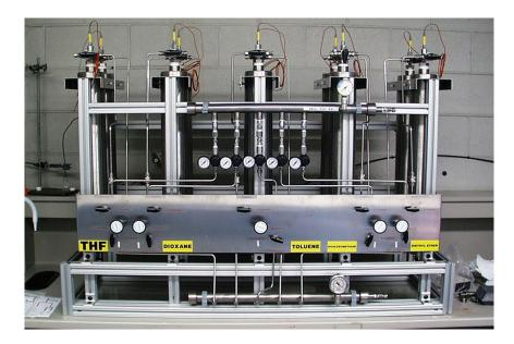
FIGURE 7.4 Example of a column purification system.
