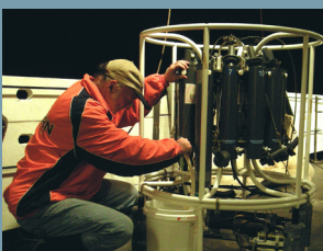
Moss collects Gulf seawater from a Niskin bottle rosette, a deepwater collection device dropped overboard and recovered on board ship.
