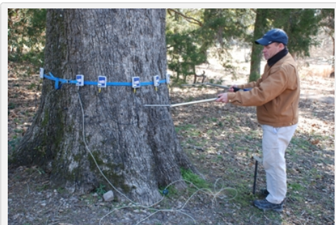
Master Arborist Chris Hastings takes a sonic scan of the Founder's Oak.
