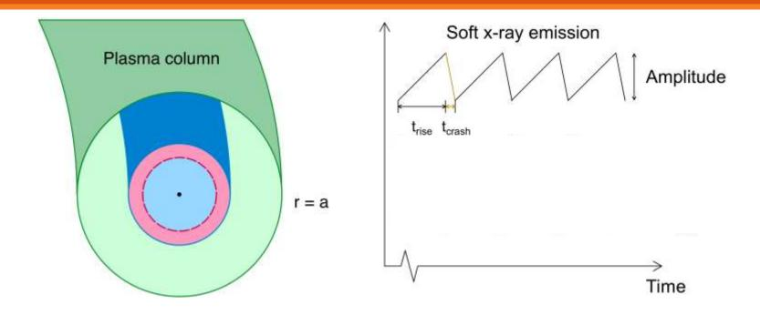
• Mechanism responsible for the sawtooth crash is instability of the m/n=1/1 internal kink/tearing mode when  $q_0 < 1$
