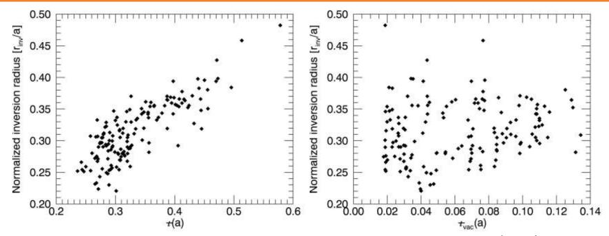
• Normalized sawtooth inversion radius is proportional to  $t(a) = 1/q(a)^1$
