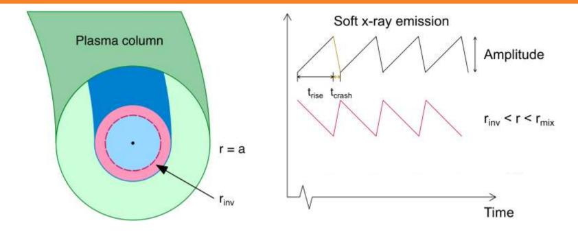
• Core plasma thermal energy inside the q=1 inversion surface is rapidly transported and deposited outside of the inversion surface due to magnetic reconnection
