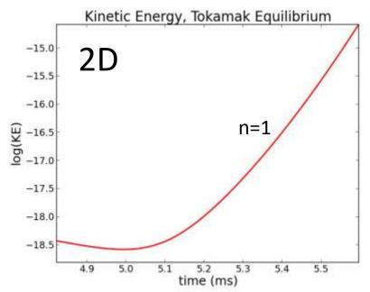
For the axisymmetric case a single growing n = 1 mode is observed
