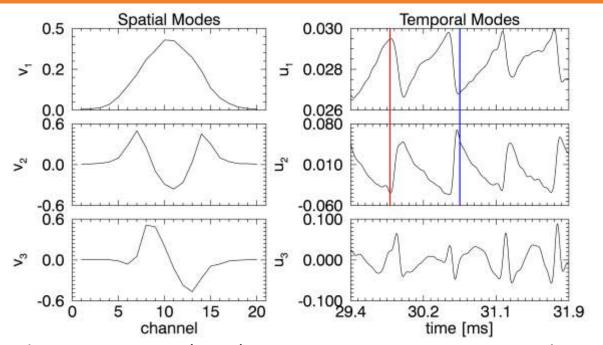
• Singular value decomposition (SVD) separates a spatio-temporal signal into two functions dependent on time or space:  $f(x,t) = \sum_n A_n v_n(x) u_n(t)$
