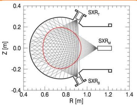
• The midplane  $SXR_M$  camera is used as an emissivity diagnostic to characterize sawtooth behavior with 3D shaping
