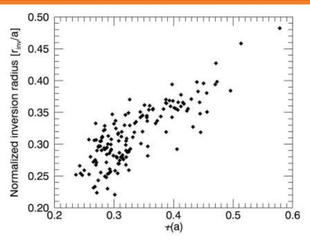
• Normalized sawtooth inversion radius is proportional to  $t(a) = 1/q(a)^1$
