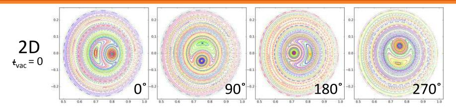
Axisymmetric plasma simulated with similar parameters to CTH
