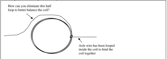
However it is important to balance the coil as much as possible. The loose length of wire shown in the diagram above will form a half loop and cause the coil to be unbalanced. Can you think of a way to re-route the length of wire that will result in a more balanced coil? As, you bind the coil, do it carefully and neatly such that you will be able to trace the direction the current will flow.
