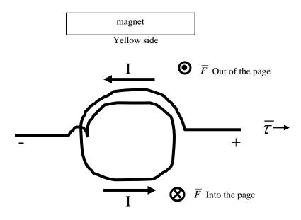
From this diagram you should be able to determine that the top of the coil is coming out of the page, and the bottom of the coil is going into the page. Applying  $\overline{F} = I\overline{L} \times \overline{B}$  at the very top and very bottom of the coil, it can be determined that the magnetic field,  $\overline{B}$ , supplied by the magnet is pointing down; therefore, the yellow side of the magnet is the North Pole of the magnet.
