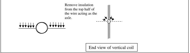
With the axles horizontal and the coil held in a vertical position, carefully remove the top half of the insulation from each axle using the rotary tool with a sanding drum attachment. Carefully guide the rotary tool to remove the insulation around half of the circumference. Excessive pressure will cause the axle to curve and wind around the sanding drum. It is important to remove the insulation from the same 'top' side on both axles. Otherwise, current will not flow.
