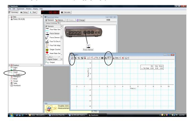
Click on the button to add the Min, Max, and Mean values to the graph. The button can be used to automatically scale the axis of the graph after you have collected data.
